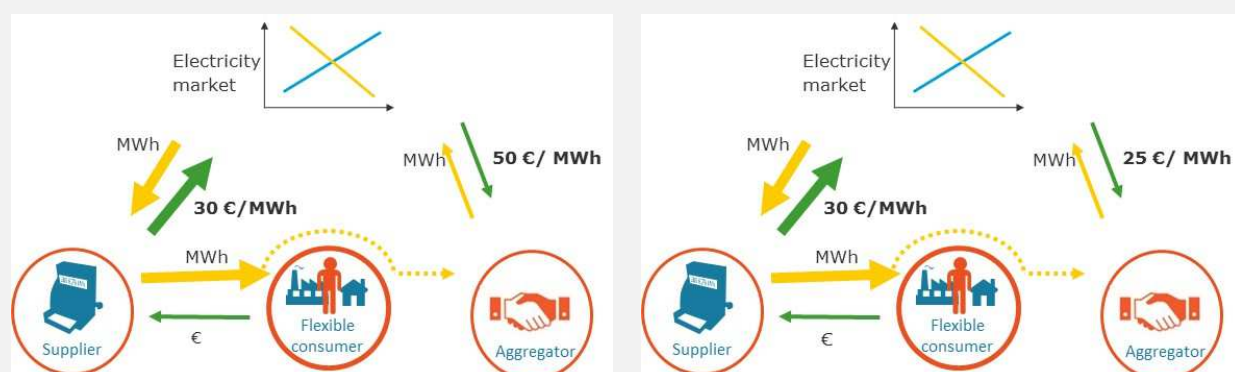
Figure 6: Illustration of the Economic Efficiency and Inefficiency of DR Depending on the Price at which DR is Activated and Energy is Procured by the Supplier
